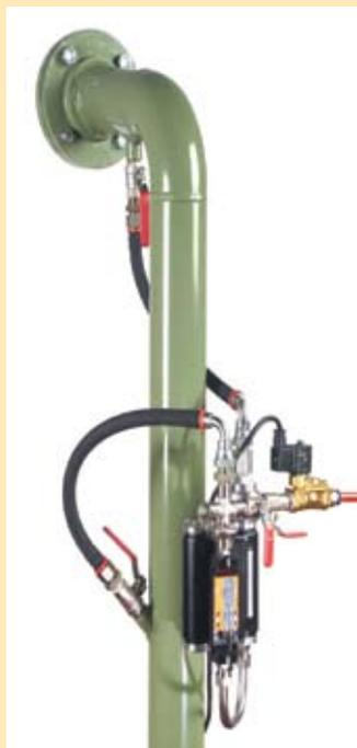
\* While ferrous debris sensors might not be effective for two-cycle cylinder regions, for the standard notion of monitoring a circulating oil, there are applications that feature individual ferrous debris sensors within each power cylinder. An example is shown in this marine installation involving very large two-cycle engine types.
