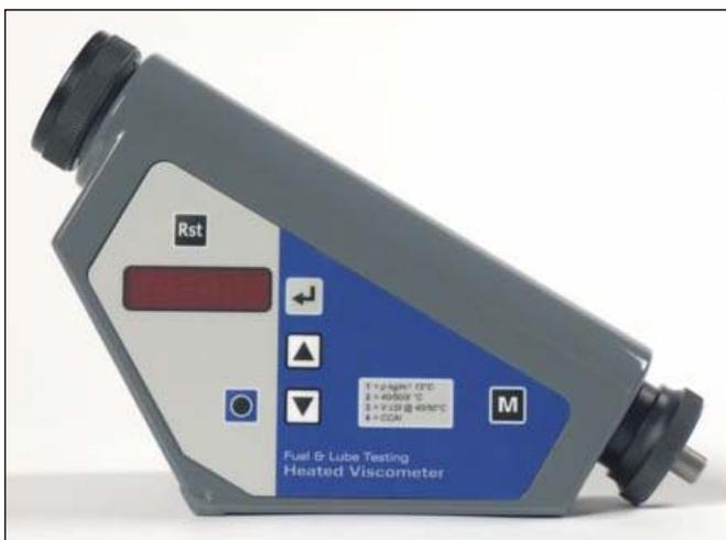
Tier 2 (onsite) Test: Electronic Viscosity test. (Courtesy of Kittiwake Developments LTD)
