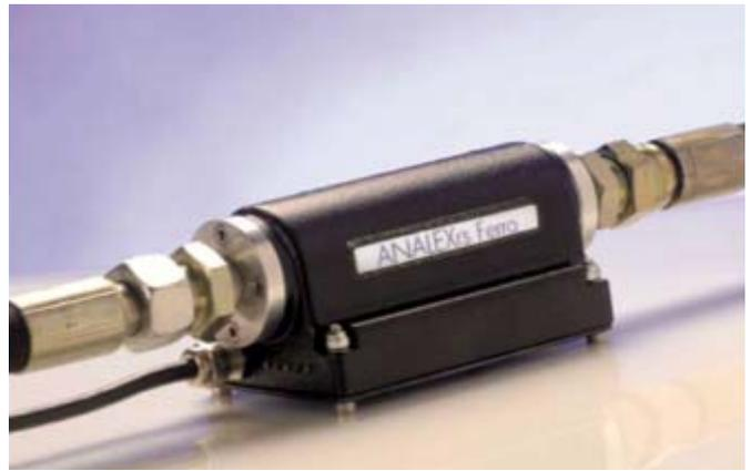
Tier 1 (online): Ferrous Particle Counter - sensitivity to 40 μ diameter. (Courtesy of Kittiwake Developments LTD)
