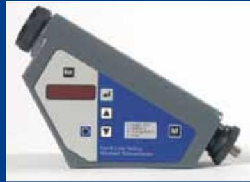
**Electronic Viscosity test for Tier 2 (onsite) Test.** *[Photo courtesy of Kittiwake Developments LTD.]*
