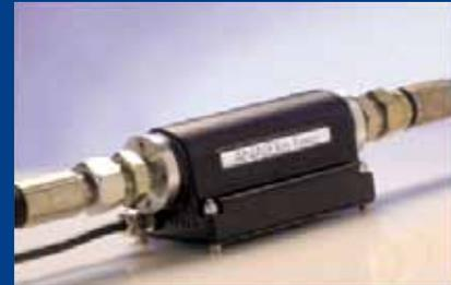
**Ferrous Particle Counter for Tier 1 (online) test.** Counter sensitivity to 40µ diameter. *[Photo courtesy of Kittiwake Developments LTD.]*
