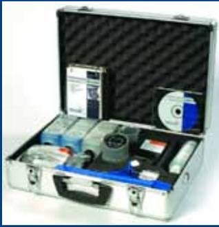
**Water-in-Oil Test Kit for Tier 2 (onsite).** *[Photo courtesy of Kittiwake Developments LTD.]*
