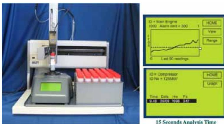
Figure 1 | Ferrous debris analyzer. [Courtesy of Kittiwake Developments Ltd.]
